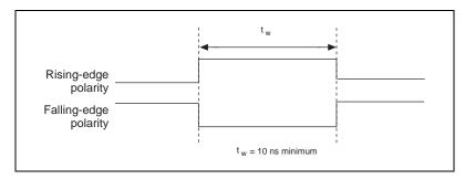
Figure 4-30. GPCTR0\_GATE Signal Timing in Edge-Detection Mode
