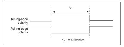
Figure 4-17. TRIG2 Input Signal Timing
