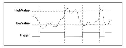
**Figure 3-9.** Low-Hysteresis Analog Triggering Mode
