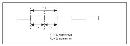
Figure 4-28. UISOURCE Signal Timing
