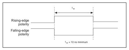
Figure 4-26. UPDATE\* Input Signal Timing
