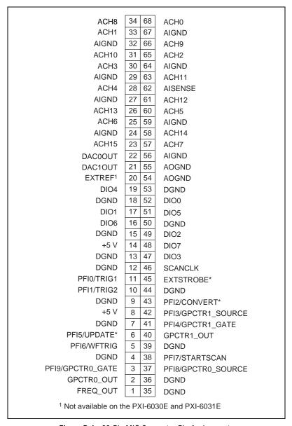
Figure B-1. 68-Pin MIO Connector Pin Assignments
