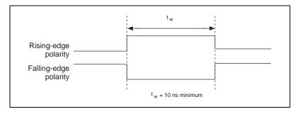
Figure 4-15. TRIG1 Input Signal Timing
