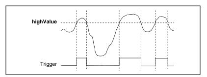
Figure 3-6. Above-High-Level Analog Triggering Mode
