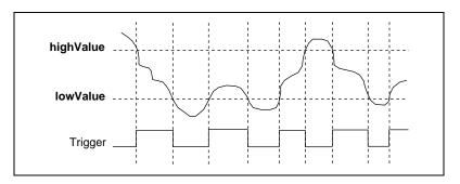
Figure 3-7. Inside-Region Analog Triggering Mode
