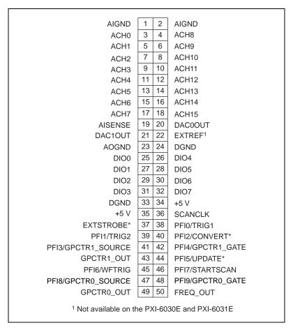
Figure B-3. 50-Pin MIO Connector Pin Assignments
