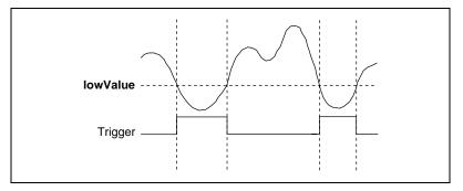
Figure 3-5. Below-Low-Level Analog Triggering Mode
