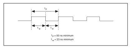
Figure 4-29. GPCTR0\_SOURCE Signal Timing
