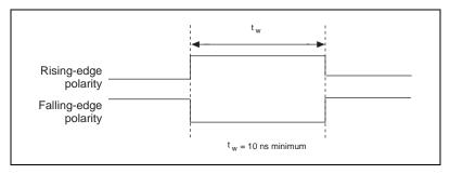
Figure 4-19. STARTSCAN Input Signal Timing
