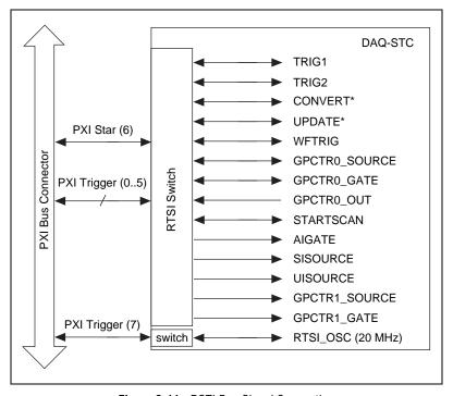
Figure 3-11. RSTI Bus Signal Connection
