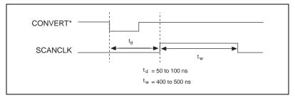
Figure 4-13. SCANCLK Signal Timing
