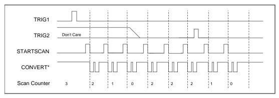
Figure 4-12. Typical Pretriggered Acquisition
