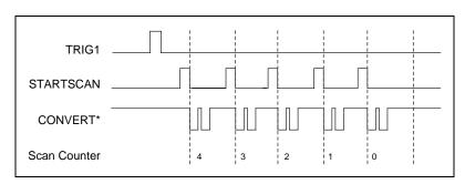
Figure 4-11. Typical Posttriggered Acquisition
