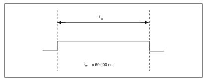
Figure 4-16. TRIG1 Output Signal Timing
