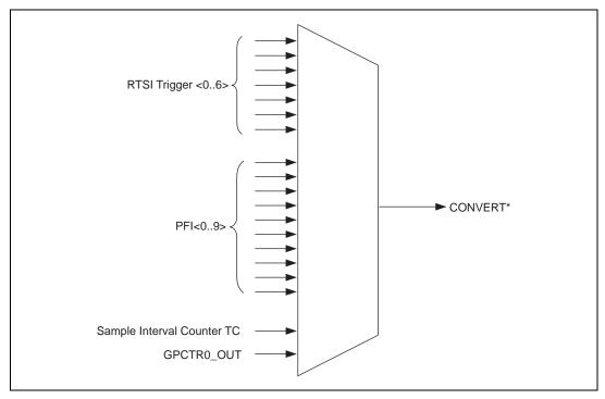
Figure 3-10. CONVERT\* Signal Routing
