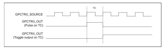
Figure 4-31. GPCTR0\_OUT Signal Timing
