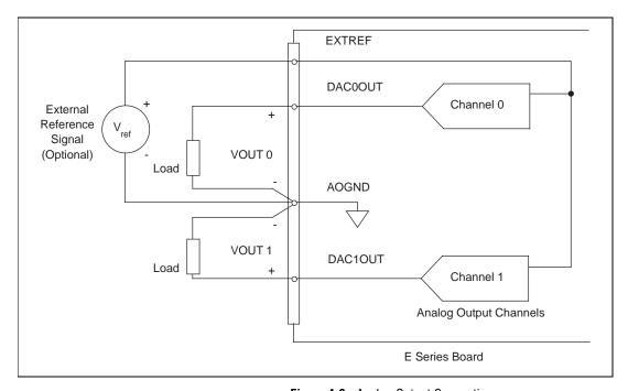
Figure 4-8. Analog Output Connections
