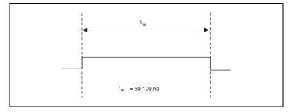
Figure 4-22. CONVERT\* Output Signal Timing
