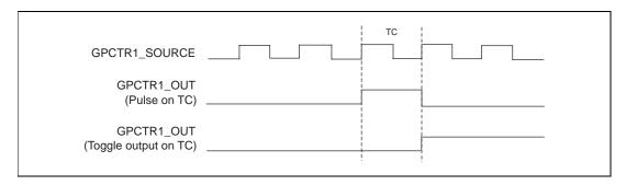
Figure 4-34. GPCTR1\_OUT Signal Timing
