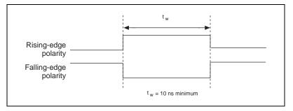
Figure 4-24. WFTRIG Input Signal Timing
