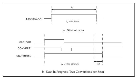
Figure 4-20. STARTSCAN Output Signal Timing
