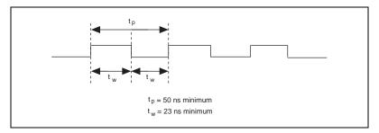
Figure 4-32. GPCTR1\_SOURCE Signal Timing
