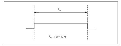
Figure 4-25. WFTRIG Output Signal Timing
