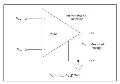
Figure 4-3. PXI E Series PGIA
