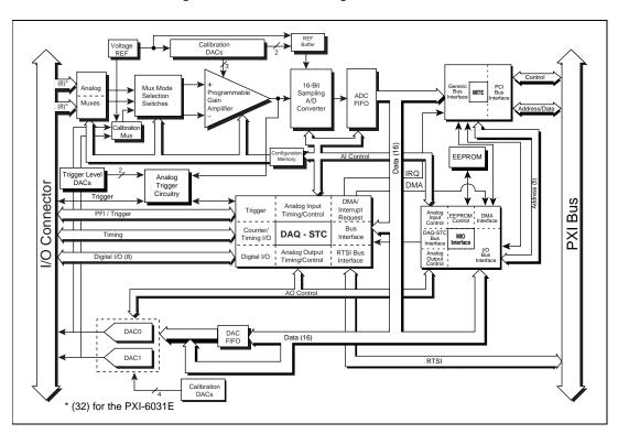
Figure 3-2 shows a block diagram for the PXI-6030E and PXI-6031E.
