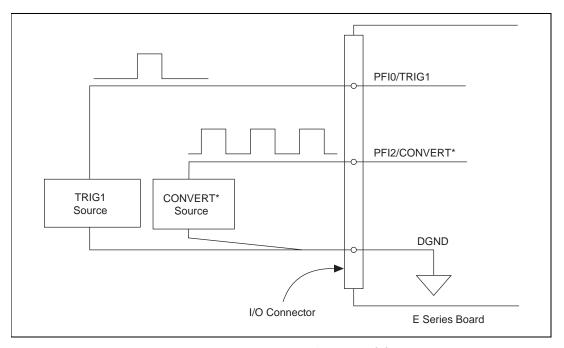
Figure 4-10. Timing I/O Connections
