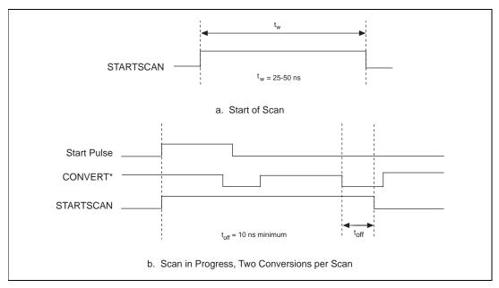
Figure 4-21. CONVERT\* Input Signal Timing
