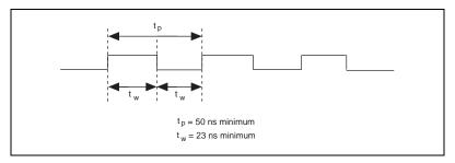
Figure 4-23. SISOURCE Signal Timing
