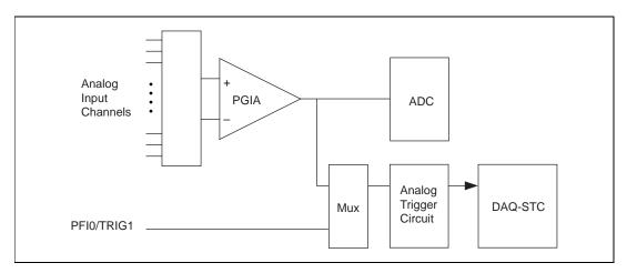
Figure 3-4. Analog Trigger Block Diagram
