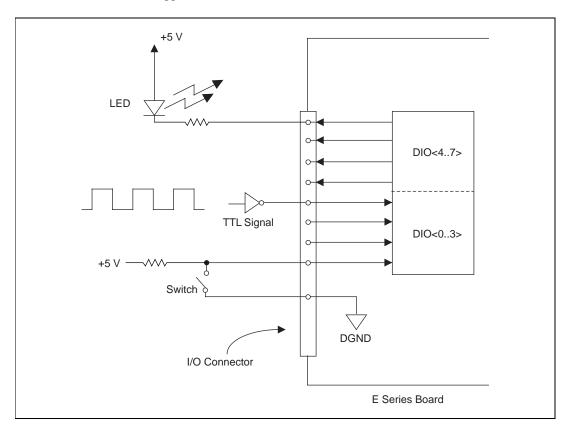
Figure 4-9. Digital I/O Connections
