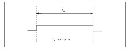
Figure 4-18. TRIG2 Output Signal Timing
