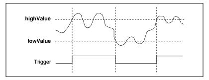
Figure 3-8. High-Hysteresis Analog Triggering Mode
